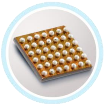
WLCSP Wafer Level Chip Scale Package (Fan-In)
